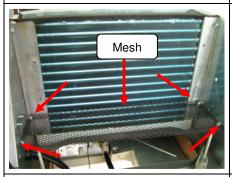
Install mesh screen (reinstall screws from step 3 and add (2) additional screws in locations shown).
