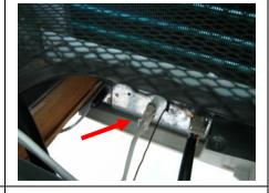
6. Connect the 3-pin connector to the control box, if installed.
