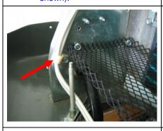
7. Secure heater lead with wire holder, as shown.
